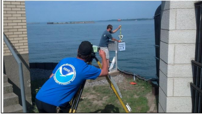
Leveling backsight to leveling point and barcode rod
