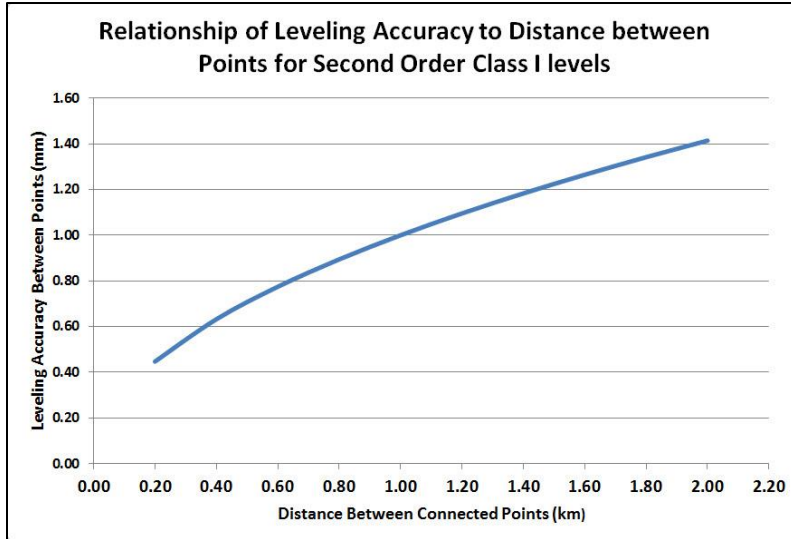
Figure 3. Leveling accuracy changes with distance
